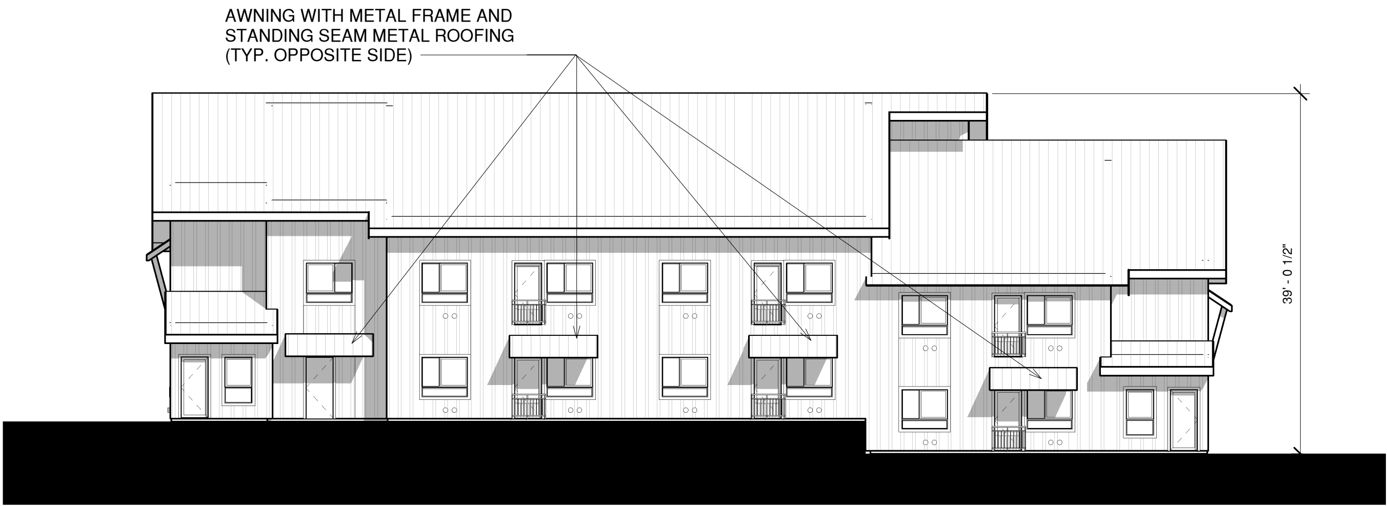
1 BUILDING C - NORTH ELEVATION 3/32" = 1'-0"
